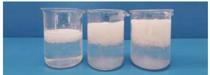
Pic. 2 Gel Raft in 0.1 M HCl, with Two, Three and Four Chewable Tablets Composed of VIVAPHARM® Sodium Alginate PH R5
